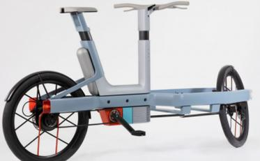
**Fun technology fact:** Researchers at the University of New South Wales have created a compact modular hydrogen-powered bicycle without the use of heavy batteries, particulates, or CO2 emissions. The LAVO bike fully charges in about ten minutes and has a range of about 93 miles (150 km). Compared to competitors, LAVO's technology has 3X the storage capacity and 2X the lifespan. Read [more of the article here](#). Price tag? The article did not say, but I would bet it is salty.
